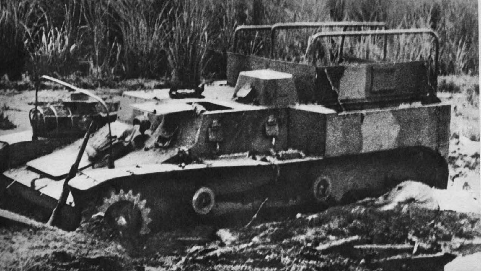
ARMORED PRIME MOVER ON POSSIBLE TANKETTE CHASSIS CARRIES MEN AND SUPPLIES IN THE REAR. SIDE PORTS ARE FOR SMALL ARMS WEAPONS
